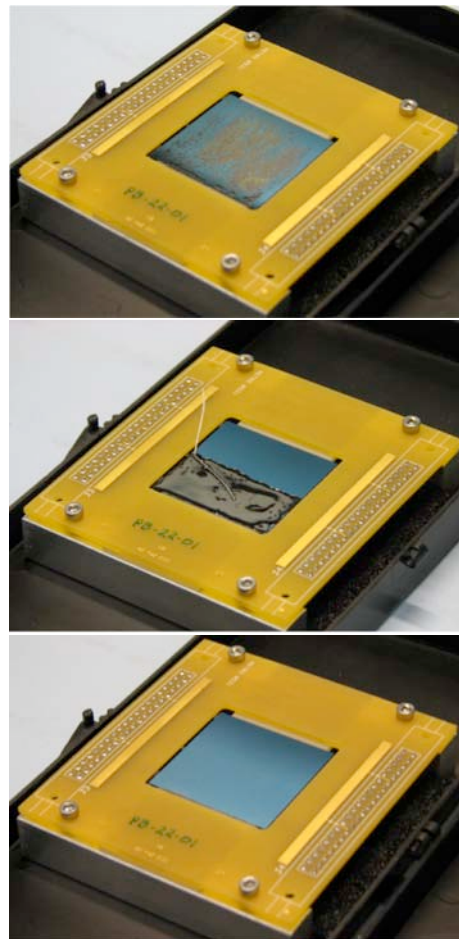
FIG. 2: Cleaning of the DECam 2x2 picture frame CCD. Top) Detector after losing vacuum while cold, Middle) Detector being cleaned and Bottom) result for the cleaning process.
