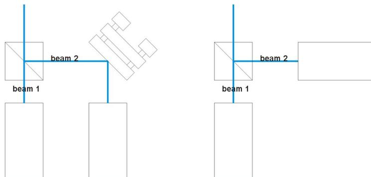
adjustable mount. This then allows for some inaccuracy of the diode mount and gives us some means of adjusting the near field alignment. Without this (as in the right image) the near field alignment will have to be done by means of positioning of the PBS cube.
