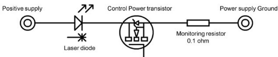
Should you wish to operate a number of diodes in series and the voltage across them would be greater than the power supply to the board you can use a higher voltage supply to the laser diodes as long as the supply to the driver and the diodes have a good common ground connection (see diagram right).
