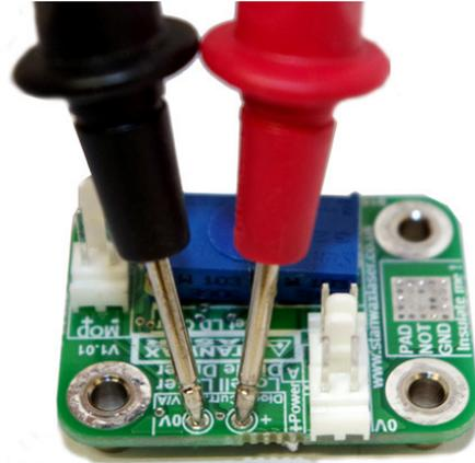
Using the test points to measure the laser diode current
