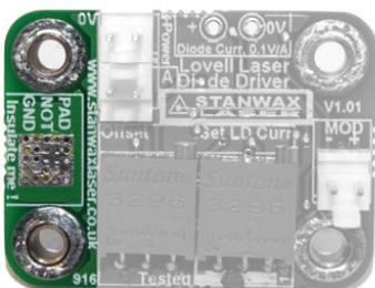
If the pad is attached to a heatsink that is not 'free standing' and is connected to the equipment grounded chassis then this pad **MUST** be insulated, using a silicone or mica pad that will provide good thermal conductivity while keeping the pad electrically isolated. Failure to do this will place the full supply voltage to the board across your laser diode and will kill it instantly.
