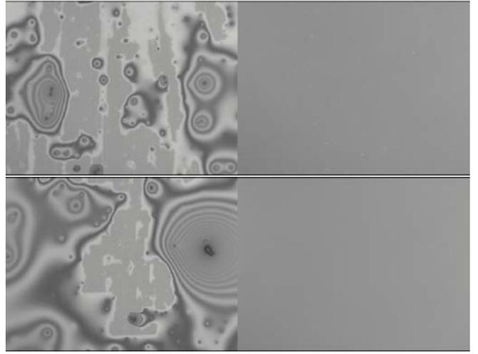
FIG. 6: Results of cleaning with acetone (top) and with *First Contact*<sup>TM</sup> (bottom) on the bulk (central region) of the CCD imager. The left images are before cleaning; the images on the right are after cleaning. After the acetone cleaning one can see some contamination as white features in the image, that are completely removed with *First Contact*<sup>TM</sup>.
