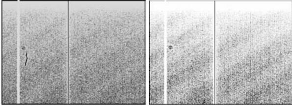
FIG. 4: 300 pixel wide region of a CCD image before (left) and after (right) cleaning with *First Contact*<sup>TM</sup>. A small fiber is efficiently removed from the surface during the cleaning process. Each pixel is  $15\ \mu\text{m} \times 15\ \mu\text{m}$ . Both images shows a hot column and a blocked column. These are produced by cosmetic defects in the Si.
