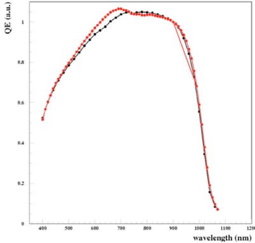
FIG. 5: Relative Quantum Efficiency measurement before (black) and after (red) cleaning with *First Contact*<sup>TM</sup>. There is no evidence of any degradation in the AR coating after the cleaning.
