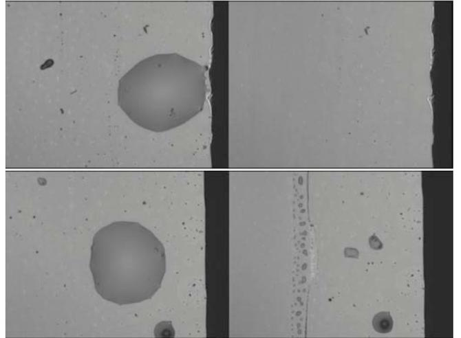
FIG. 7: Results of cleaning with acetone (top) and with *First Contact*<sup>TM</sup> (bottom) on the edge of the CCD imager. The left images are before cleaning; the images on the right are after cleaning. The application of *First Contact*<sup>TM</sup> to the edge of the detector is difficult and some residue remains compared with the acetone swab.
