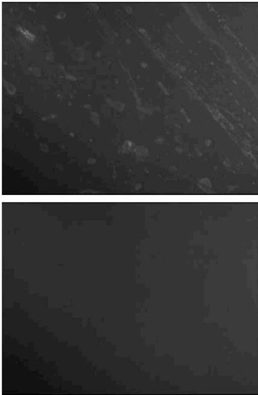
FIG. 3: Microscopic images of a wafer after cleaned with acetone (top) and after the application of *First Contact*<sup>TM</sup> (bottom). The image width is  $\sim 340 \mu\text{m}$ .
