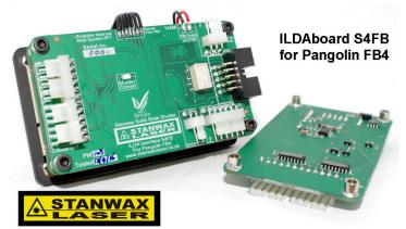
The most significant feature on the S4 version of our widely used ILDA board is the addition of \*Stanwax Solid State Shutter technology – hence the name S4. This provides a six channel electronic shutter that will kill laser output via the laser modulation lines in <100uS. This has been developed and tested over a number of years so we are confident that you will have the safest and most compliant laser projector yet with this system.
