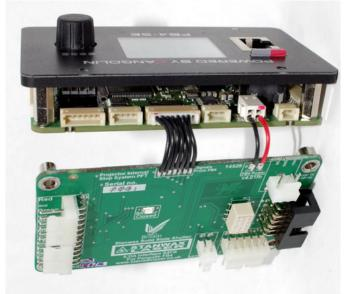
Fit the 8 way connector from the ILDA board to the header and push the red and black power wires into the receptacles on the FB4 ensuring correct polarity. Press the red and black wires firmly into the receptacle to ensure a good connection.
