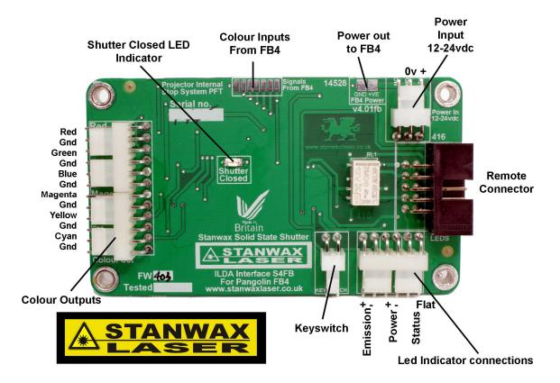
Power connection – 12-24VDC (note the connector has an unused pin and is provided with 3 pins to be 100% compatible with other versions of this product) Looking from the top Right Pin +Ve Centre pin 0v Left pin NC
