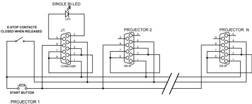
As you can see the connector for projector 1 has the e-stop and start button contacts as well as the laser status Bi-Coloured LED connected to it, the others need only have pins 1, 4 and 8 from the 9 pin connector linked between projectors. Also note that connecting via the interlock loops the e-stop function is independent of the ILDA inputs so it does not matter if the projectors are running of one laser controller or several, the e-stop and start function will still work.
